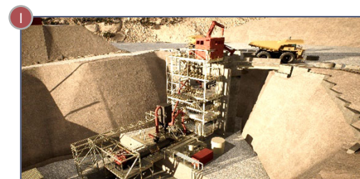
Crushing circuit, including two HPGR units (capacity of ~28.5M tons/year)
